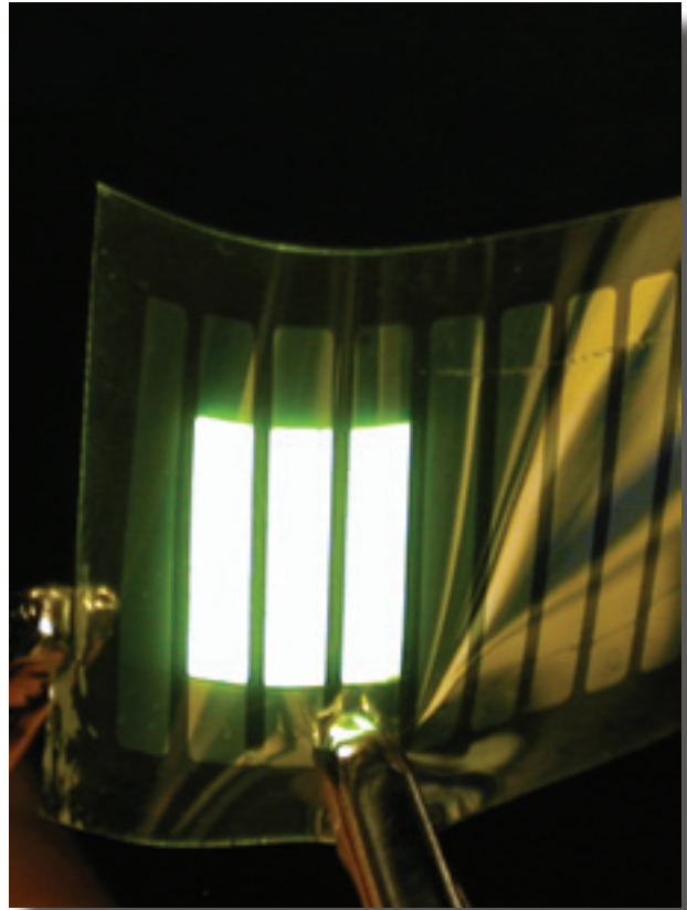
Flexible polymer light emitting diodes developed at Imperial College London using a new patterning procedure known as 'interlayer lithography'
